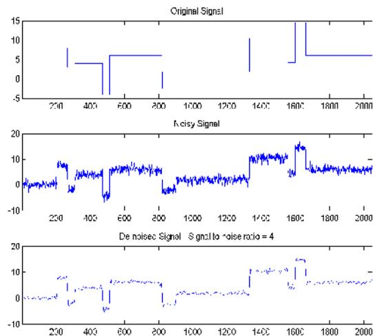
Fig. 5. Original Signal, Noisy Signal, De-noised Signal.
